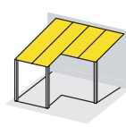
Pent roof with roof guttering offset
